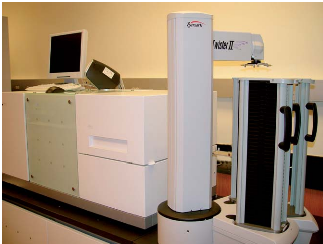
FIG. 2. Opera with Twister II plate robot and plate stacks on a Scala. An interface station with keyboard switch for the evaluation network is visible on top of the instrument.
