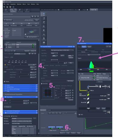
(7) **Select (+) to add a new track**Adjust the laser and detector so that Track 2 is identical to Track 1.
